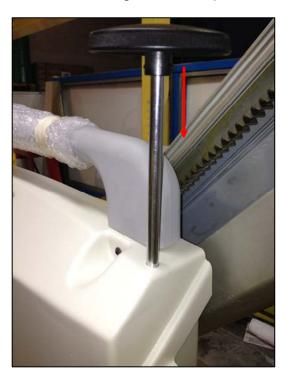
3. Whilst pushing down on the winding wheel, push the barrier arm in towards the carriage.
